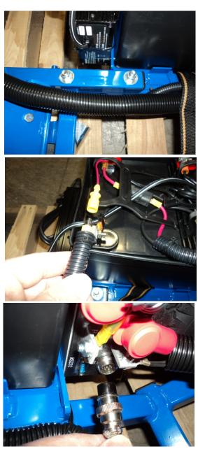
**Step 4:** Install battery box strap through and under battery box platform and tighten. You can include the wiring tube inside the battery strap as seen in picture or you can use the supplied zip ties to hold it close to the battery box so it does not interfere with the loading operation.
