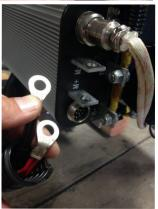
Test the leads from the motor directly to the 24V terminals firmly press one lead to either terminal, and then firmly and quickly press the other lead to the opposite 24V terminal. If you switch the leads to the opposite terminals, the transaxle will spin in the opposite direction.
